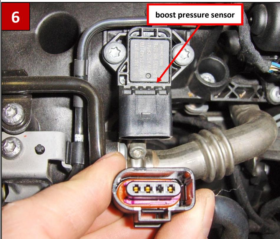
◇ Disconnect the plug from the boost pressure sensor
