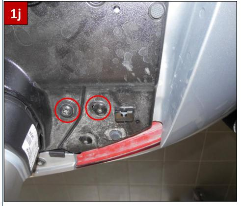
Unscrew the fixing screws of the mounting bracket of the rear spoiler along the rear bumper.
