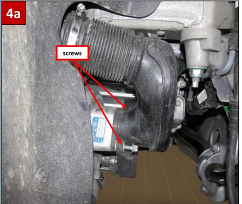
♦ Then loosen the 2 marked screws and remove the hose carefully.
