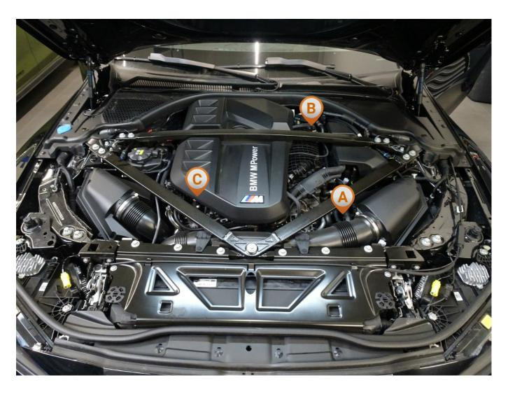
View of longitudinally mounted engine
