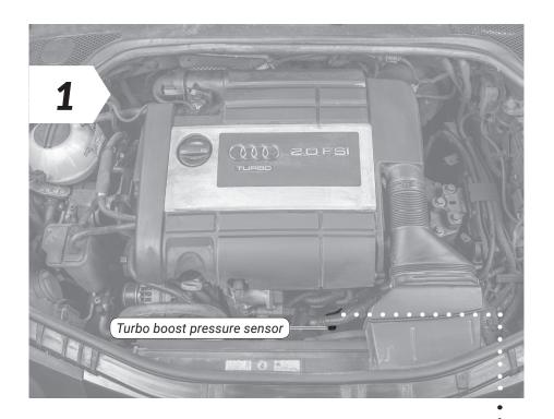
First locate the turbo boost pressure sensor connection in your engine bay.
