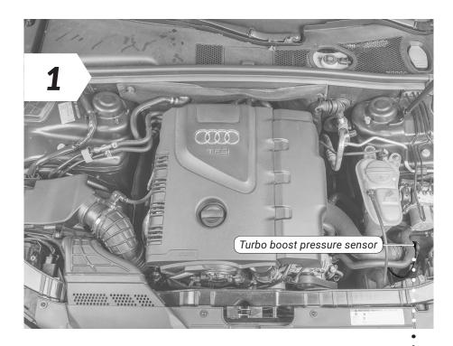
• First locate the turbo boost pressure sensor connection in your engine bay.
