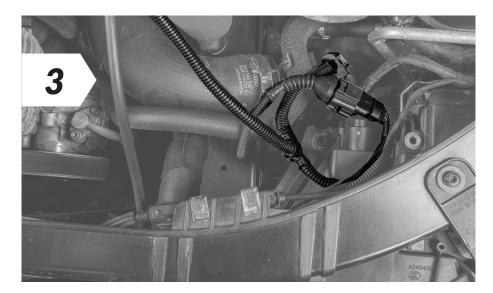
Now connect the end of the VR Tuned wiring harness to the disconnected connector and the other end to the sensor.
