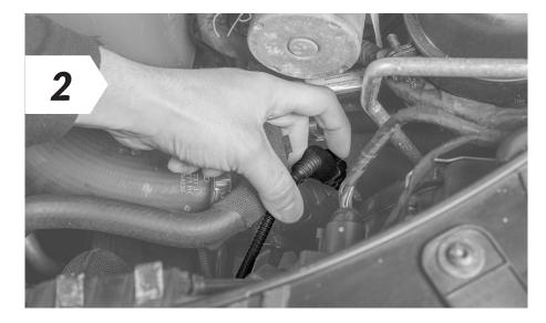
Disconnect the turbo boost pressure sensor
