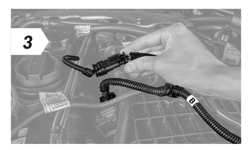
• Now connect the end of the performance upgrade wiring harness marked "**B**" to the disconnected connector and the other end to the sensor.
