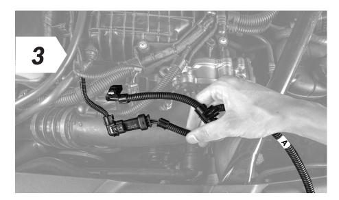
• Now connect the end of the performance upgrade wiring harness marked "**A**" to the disconnected connector and the other end to the sensor.
