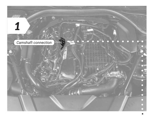
• Once the connection tto the manifold absolute pressure is complete, it is time to make the connection to the camshaft sensor.
