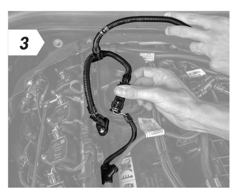
Now connect the end of the performance upgrade wiring harness marked "**C**" to the disconnected connector and the other end to the sensor.
