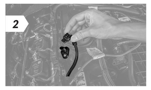
• Disconnect the plug from the camshaft sensor.
