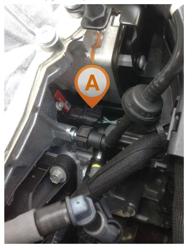
4) Please disconnect plug B and connect the male and the female plug to the female and the male plug of the RaceChip cable harness.
