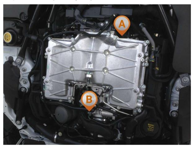
3) Please disconnect plug A and connect the male and the female plug to the female and the male plug of the RaceChip cable harness.
