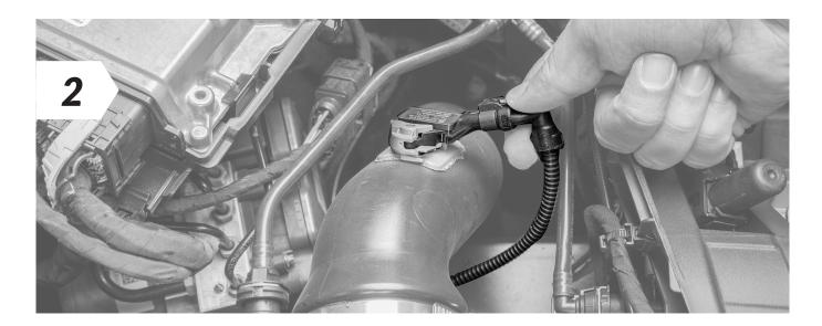
• Disconnect the turbo boost pressure sensor
