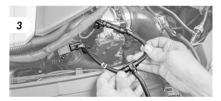
• Now connect the end of the VR Tuned wiring harness marked "B" to the disconnected connector and the other end to the sensor.
