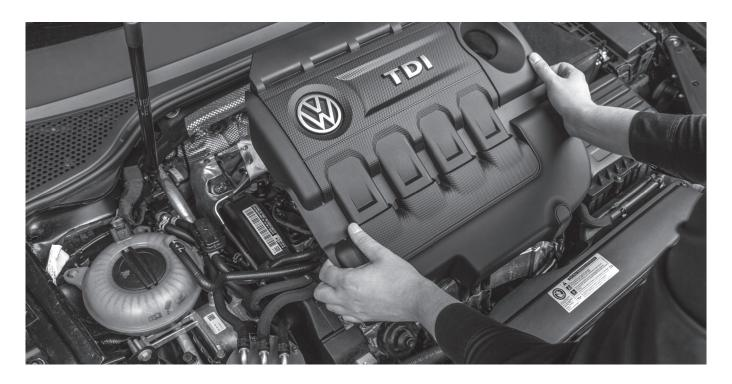
Remove the engine cover and place it next to the car. You may have to jiggle the cover slightly to release it from the holding clips.
