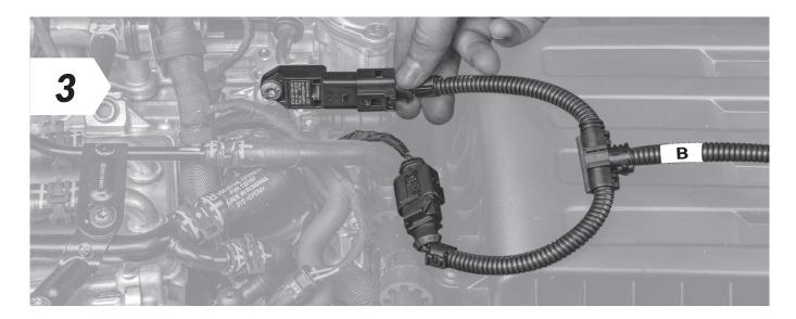
Now connect the end of the VR Tuned wiring harness marked "B" to the disconnected connector and the other end to the sensor.
