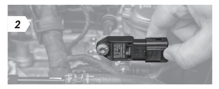
· Disconnect the turbo boost pressure sensor
