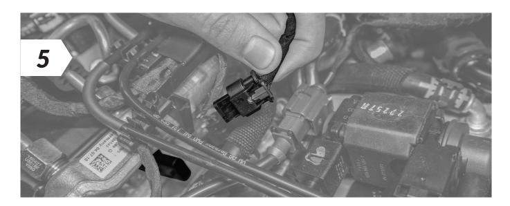
Disconnect the plug from the camshaft sensor.
