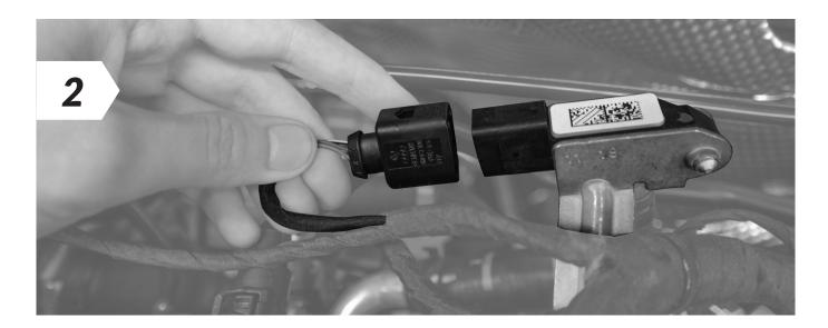
Disconnect the turbo boost pressure sensor
