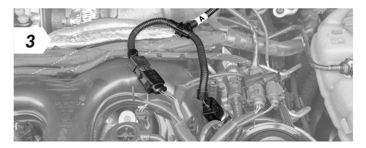
Now connect the end of the VR Tuned wiring harness to the disconnected connector and the other end to the sensor.
