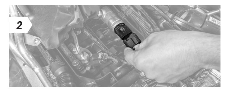
• Disconnect the plug from the common rail sensor.
