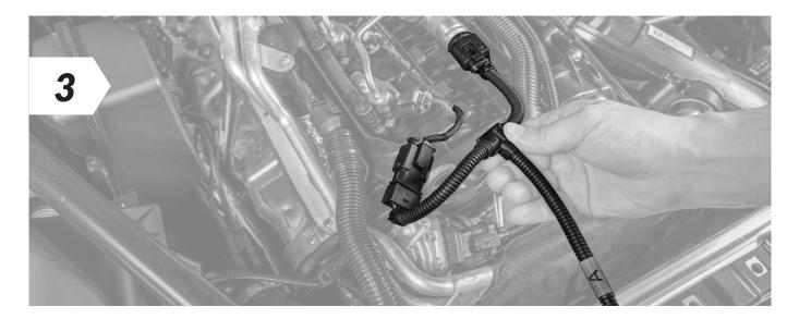
• Now connect the end of the VR Tuned wiring harness marked "A" to the disconnected connector and the other end to the sensor.
