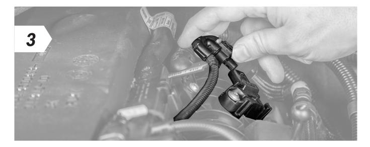
• Disconnect the turbo boost pressure sensor
