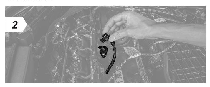
• Disconnect the plug from the camshaft sensor.
