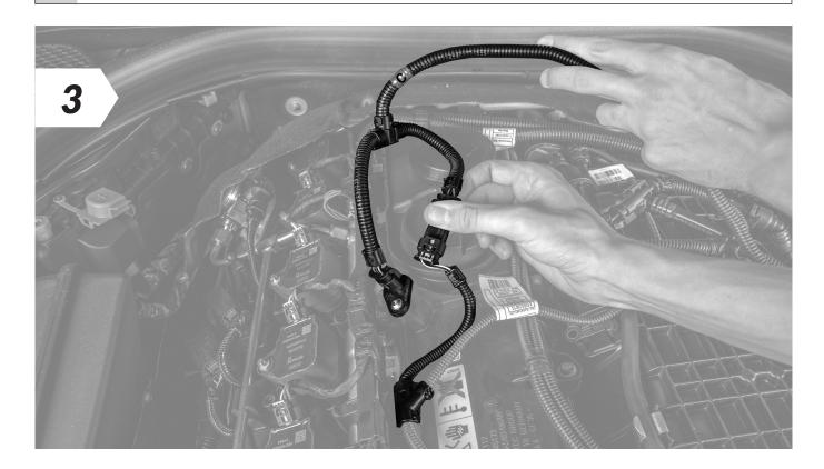
• Now connect the end of the VR Tuned wiring harness marked "C" to the disconnected connector and the other end to the sensor.
