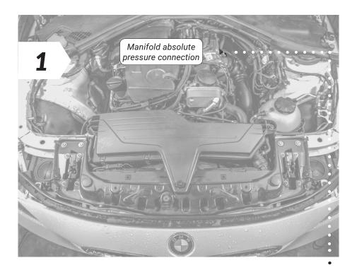
• Once the connection to the turbo boost pressure is complete, it is time to make the connection to the manifold absolute pressure sensor.
