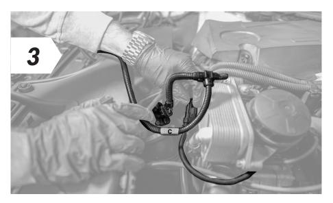
**1** Make sure that the plugs are orientated correctly to each other. If not orientated correctly, the connectors can't be connected.
