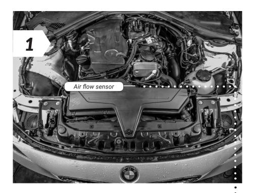
Once the connection to the Manifold absolute pressure is complete, it is time to make the connection to the air flow sensor. To begin, locate the air flow sensor in your engine bay.
