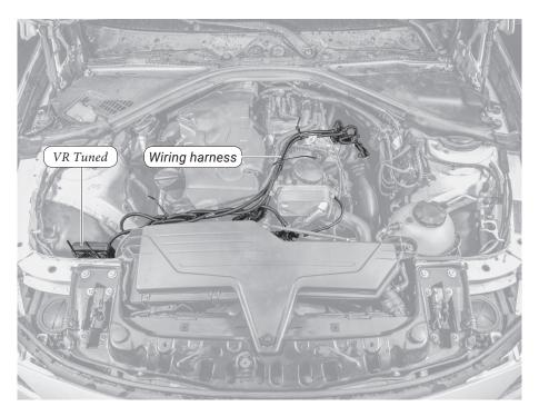
Before fixing the VR Tuned in place in the engine bay, ensure that the wiring harness can also be routed and fixed securely without putting it under excessive tension.
