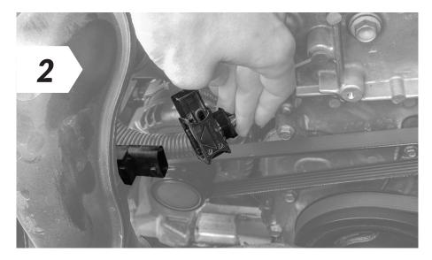
Disconnect the turbo boost pressure sensor
