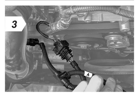
Now connect the end of the VR Tuned wiring harness marked "**A**" to the disconnected connector and the other end to the sensor.
