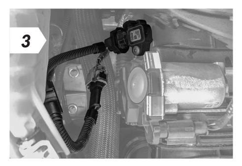
• Now connect the end of the VR Tuned wiring harness marked "**B**" to the disconnected connector and the other end to the sensor.
