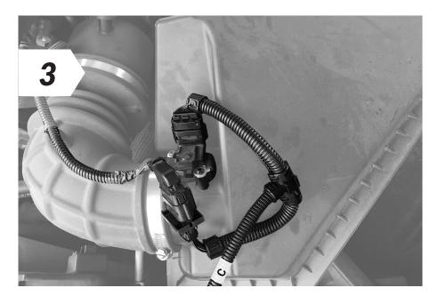
Now connect the end of the VR Tuned wiring harness marked "**C**" to the disconnected connector and the other end to the sensor.
