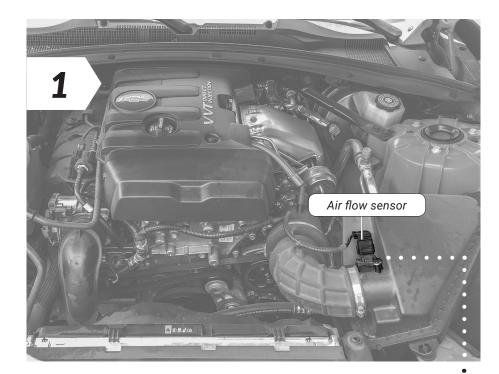
Once the connection to the manifold absolute pressure is complete, it is time to make the connection to the air flow sensor. To begin, locate the air flow sensor in your engine bay.
