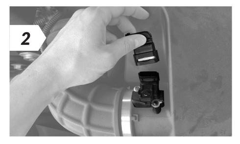
• Disconnect the air flow sensor.
