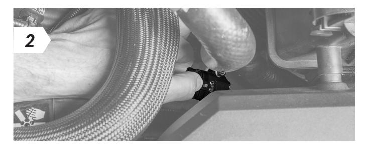
• Disconnect the turbo boost pressure sensor
