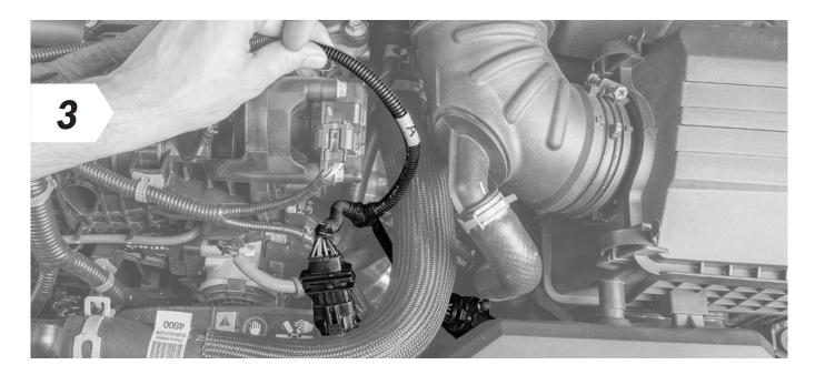
• Now connect the end of the VR Tuned wiring harness marked "A" to the disconnected connector and the other end to the sensor.
