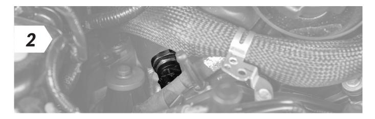
• Disconnect the plug from the common rail sensor.
