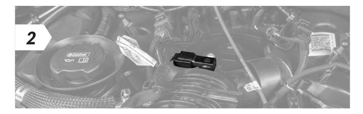
Disconnect the turbo boost pressure sensor
