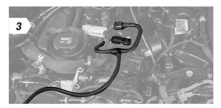
Now connect the end of the VR Tuned wiring harness marked "B" to the disconnected connector and the other end to the sensor.
