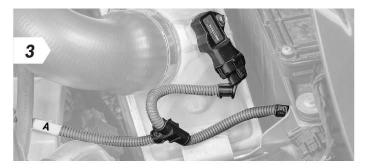
• Now connect the end of the VR Tuned wiring harness marked "A" to the disconnected connector and the other end to the sensor.
