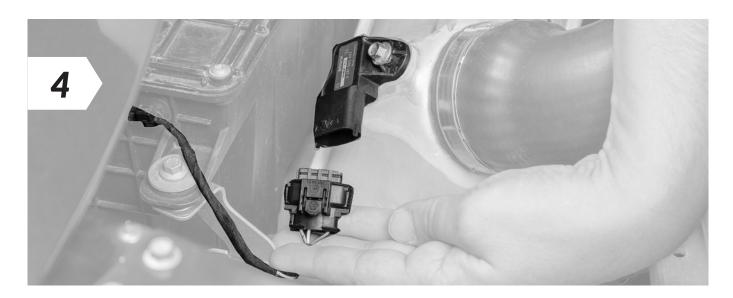
• Disconnect the turbo boost pressure sensor on the left-hand side of the engine
