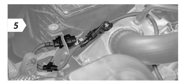
Now connect the end of the additional VR Tuned wiring harness marked "A" to the disconnected connector, and the other end to the sensor.
