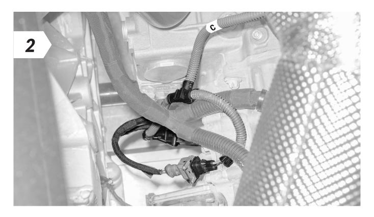
Disconnect the gearbox temperature sensor
