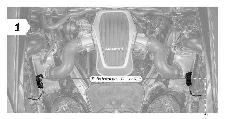
• First locate the turbo boost pressure sensor connections in the engine bay.
