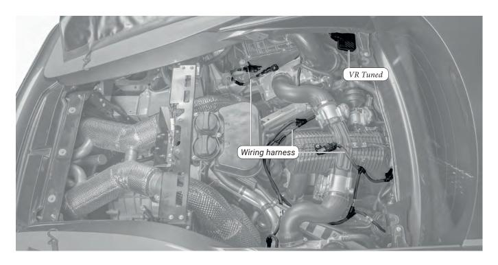
• Before fixing the VR Tuned in place in the engine bay, ensure that the wiring harness can also be routed and fixed securely without putting it under excessive tension.
