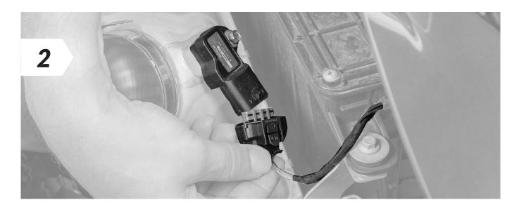
Disconnect the turbo boost pressure sensor on the right-hand side of the engine.
