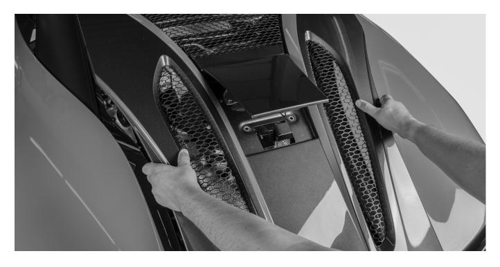
Replace the engine cover. Re it the engine compartment lid and replace the screws, tightening them carefully.
