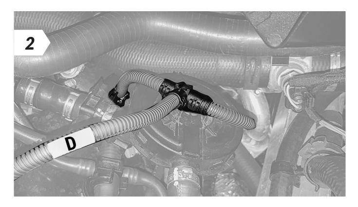
• Disconnect the plug from the camshaft sensor.
