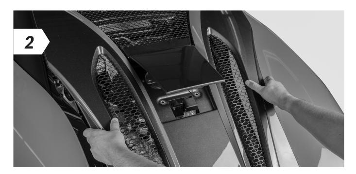
• Once the screws are undone, you can remove the engine compartment lid from its brackets, moving it gently from side to side if necessary. Place the lid in a safe location.
