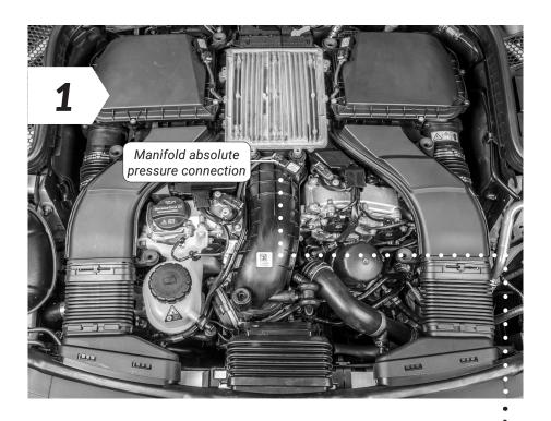
• Once the connection to the turbo boost pressure is complete, it is time to make the connection to the manifold absolute pressure sensor.
