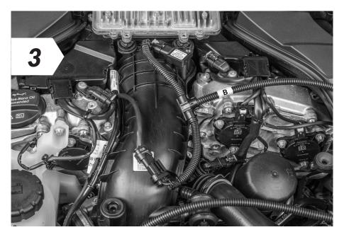
**1** Make sure that the plugs are orientated correctly to each other. If not orientated correctly, the connectors can't be connected.
