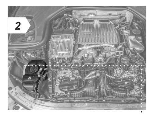
• Loosen the plastic clips on the coolant expansion tank.
