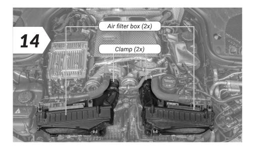
Loosen the two clamps with a screwdriver.
