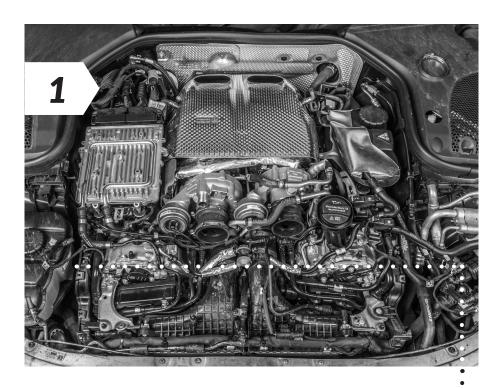
Once the connection to the turbo boost pressure is complete, make the connection to the left manifold absolute pressure sensor.
