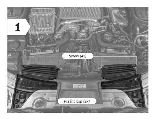
• First remove the air shroud of the air filter box.
