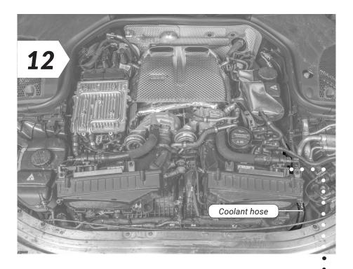
Locate the coolant hose in your engine bay, which runs along the right side of the engine.
