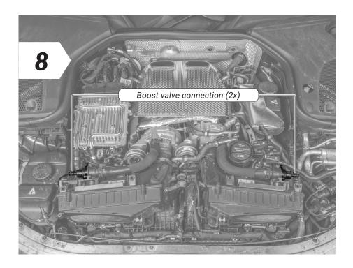
Locate the boost valve connections in your engine bay.
