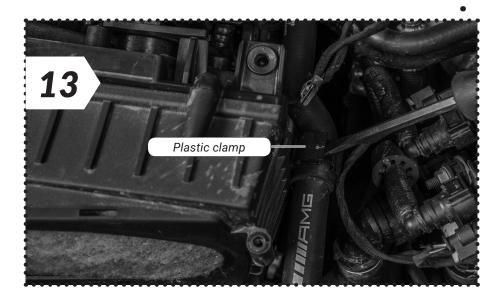
• Loosen the plastic clamp of the coolant hose.
