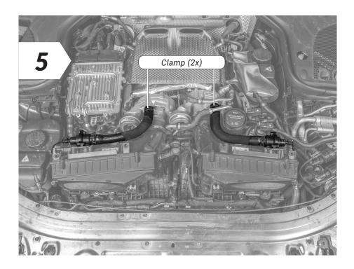
• Loosen the clamps of the boost valve with a pliers.
