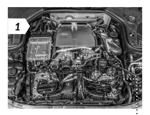
• Once the connection to the left manifold absolute pressure is complete, make the connection to the right manifold absolute pressure sensor.
