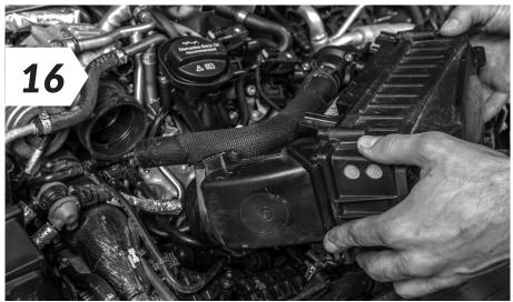
• Pull both air filter boxes out of the retaining clips and place it next to the car. You may have to jiggle the air filter box slightly to release it from the holding clips.
