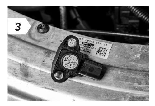
• Disconnect the right turbo boost pressure sensor
