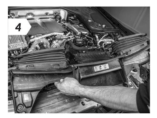
Once the screws are undone, you can remove the air shroud from its brackets.
