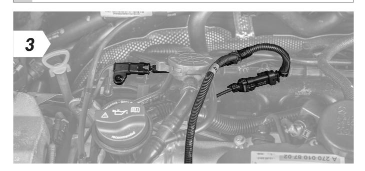
• Now connect the end of the VR Tuned wiring harness marked "B" to the disconnected connector and the other end to the sensor.
