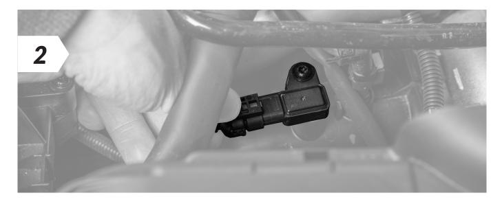
• Disconnect the turbo boost pressure sensor
