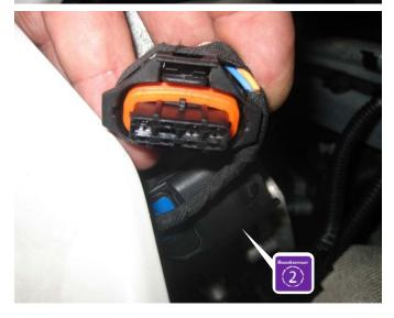
Open the plug by pressing the locking lever and connect the adapter in between both connections.
