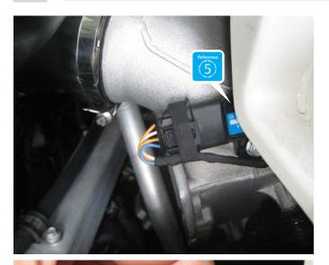
Localise the right area from the engine compartment. The boost pressure sensor is located at the pressure pipe before throttle valve.
