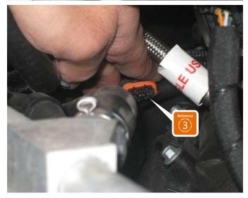
Remove the suction tube (P) to get better access to the camshaft sensor.
