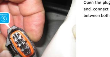
Open the plug by pulling the pressing the lever and connect the boost pressure adapter in between both connections.
